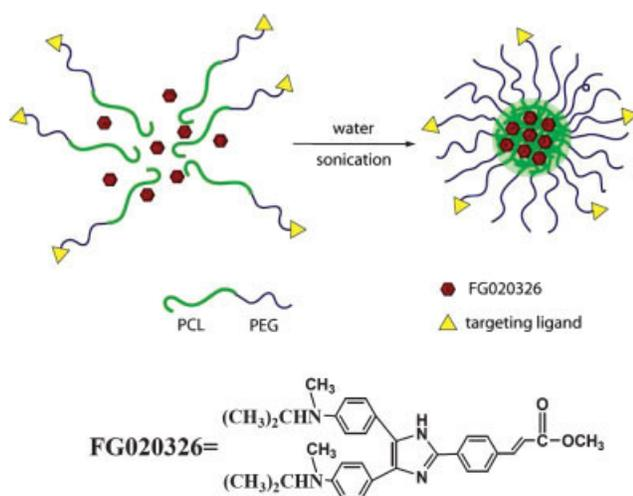
**Figure 1.** Schematic formation of FG020326-encapsulated micelle by adding THF solution containing FG020326 and copolymer to water under sonication, followed by evaporation of THF. [Color figure can be viewed in the online issue, which is available at [www.interscience.wiley.com](http://www.interscience.wiley.com).]
