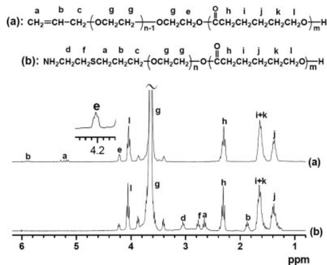
**Figure 2.**  $^1\text{H}$  NMR spectra of allyl-PEG3k-PCL1k (a) and  $\text{NH}_2$ -PEG3k-PCL1k (b) in  $\text{CDCl}_3$ . The expanded peak “e” at  $\sim 4.2$  ppm indicates the successful synthesis of block copolymer.
